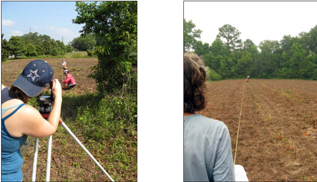
Figure 23: Grid layout in Field B, after plowing; placement of grid points with tapes
